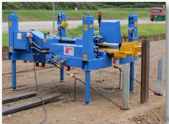
M.A.R.T.IN.A equipment, to perform of performing push tests in a quasi-static and dynamic regime on posts either driven into the ground or anchored to steel/concrete foundations
